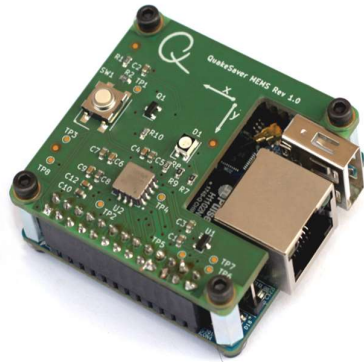
Fig 2: QuakeSaver MEMS accelerometer. (left) The bare-bones compute unit with Ethernet port for scale. (right) The sensor unit enclosure for indoor deployment in buildings.
