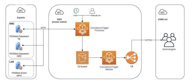
*Figure 2 - High Level Diagram (HLD) of the implementation of ObsPy's Coincidence Trigger at KNMI using the AWS platform.*
