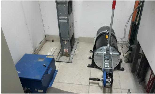
Figure 2. Use of Impact Hammer: (a) Attached to the floor, (b) Placed against a column
