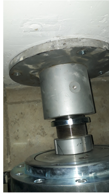
Figure 2. Use of Impact Hammer: (a) Attached to the floor, (b) Placed against a column
