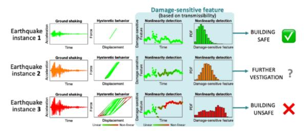
Figure: Damage-sensitive features (here transmissibility between base accelerations and rooftop accelerations) allow detecting nonlinear behaviour. Based on the distribution of the damage-sensitive feature and pre-established thresholds, the building can be tagged as safe or unsafe. Hysteretic behaviour, a direct indicator of nonlinearity, cannot be measured directly.
